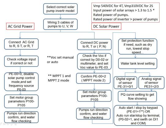
PH380 solar pump inverter operation flow chat
