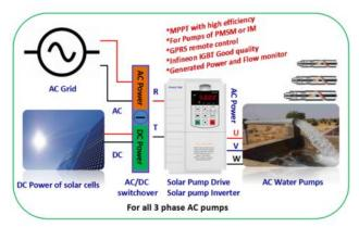
Note: Please note that polarity connecting for DC power input to P and N terminals.
