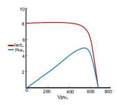
The I-V curve is not constant since intensity and temperature changes during day time. Under constant temperature, current changes linearly with intensity and voltage changes logarithmically with intensity. Since the voltage variation is small with respect to intensity changes, maximum power varies proportionally with intensity
