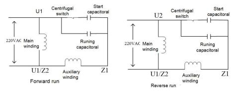
Single-phase motor is mainly composed of main winding (U1 / U2), auxiliary winding (Z1 / Z2), running capacitor, starting capacitor, centrifugal switch;
