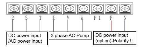
Fig 5.3-3. 3 phase AC power input for above 30 kw inverter
