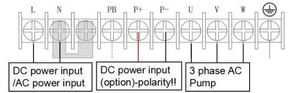
Fig 5.3-1. 1 phase AC power input 220V main circuit loop connection
