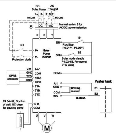
PH380 solar pump wiring 2, digital switch for water tank fulling
