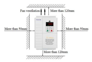
Solar pump inverter installation space requirement.
